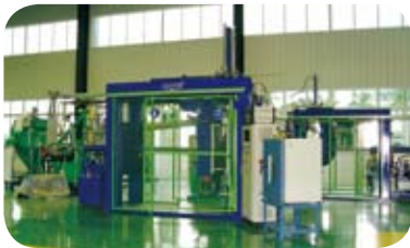
CNC epoxy resin pressure molding
